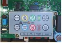
Press the transmitter button you would like to use to control the door for two seconds - Release and pause for two seconds - Press the same button again for two seconds - Release the **Door Code** or **SW1** button - Press the transmitter button to test operation of the door/gate etc Repeat for light using LIGHT CODE & A spare button **Note:** To remove a transmitter's code from the device repeat steps 1-5 above.
