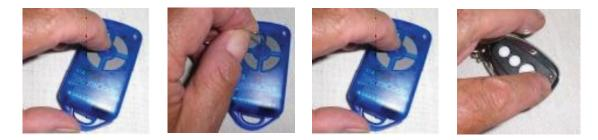
Then using a small pin or paperclip - press through the centre hole of the **Working Remote** and hold firmly for two seconds - Within 10 seconds take the **New Remote** you wish to code - Press the button you would like to use to control the device for two seconds - Pause for two seconds then press the same button again for two seconds. This button should now be coded. - Wait for 10 seconds and then press the **New Remote** button to confirm that it operates the door/gate etc.
